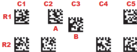
Symbol A is part of C2 if Minimum Same-Column Symbol Overlap Width Percentage is set to 20.
